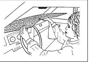
2 With both hands, lift the top of the Sunshield into the windshield area. (Be sure not to bend corners while installing, or damage to the inner insulator may occur.)
